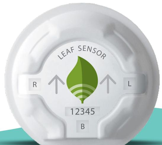
The sensor takes measurements of the patient's orientation and communicates this data wirelessly to the mesh network of LEAF Relay Antennas that had previously been setup in the facility.
